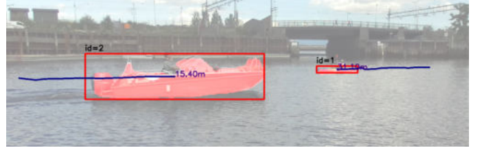
Fig. 1. Tracking visualized in the image coordinate system. The target boat and kayak are detected by YOLOv8 and tracked by BoT-SORT. The navy blue line illustrates the previous tracks of the object in the image coordinate system.
