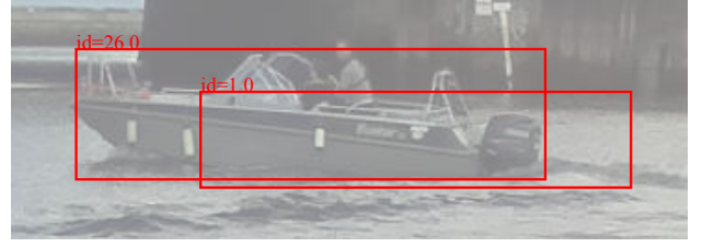
Fig. 7. Demonstration of an ID-switch: The target boat was undetected for several frames, leading to the SORT algorithm assigning a new ID to the track, changing it from 1 to 26.
